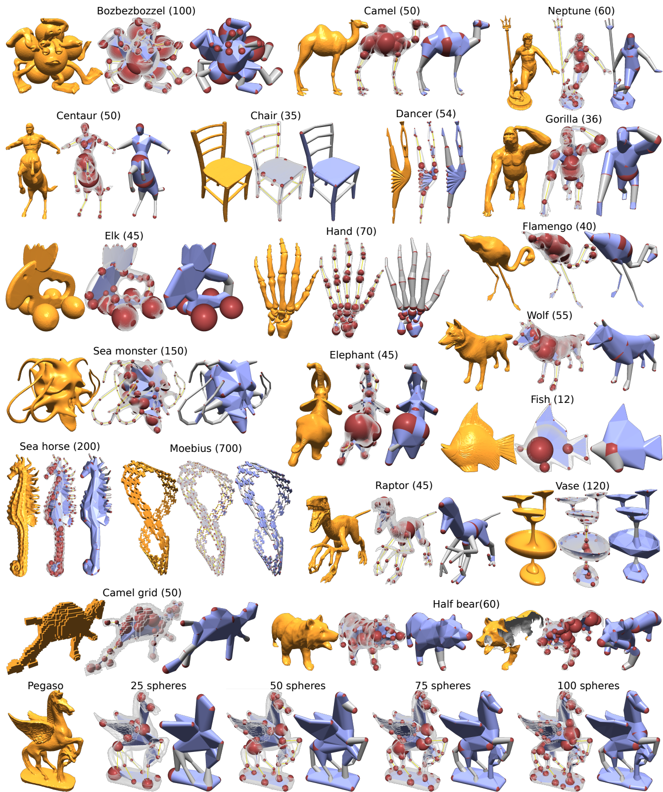
Figure 5: Sphere-mesh approximation results with the algorithm described in Sec. 3 on various meshes at different levels of simplification. Results obtained with \sigma = 1 . The number of spheres of the approximation is shown between the parentheses.
