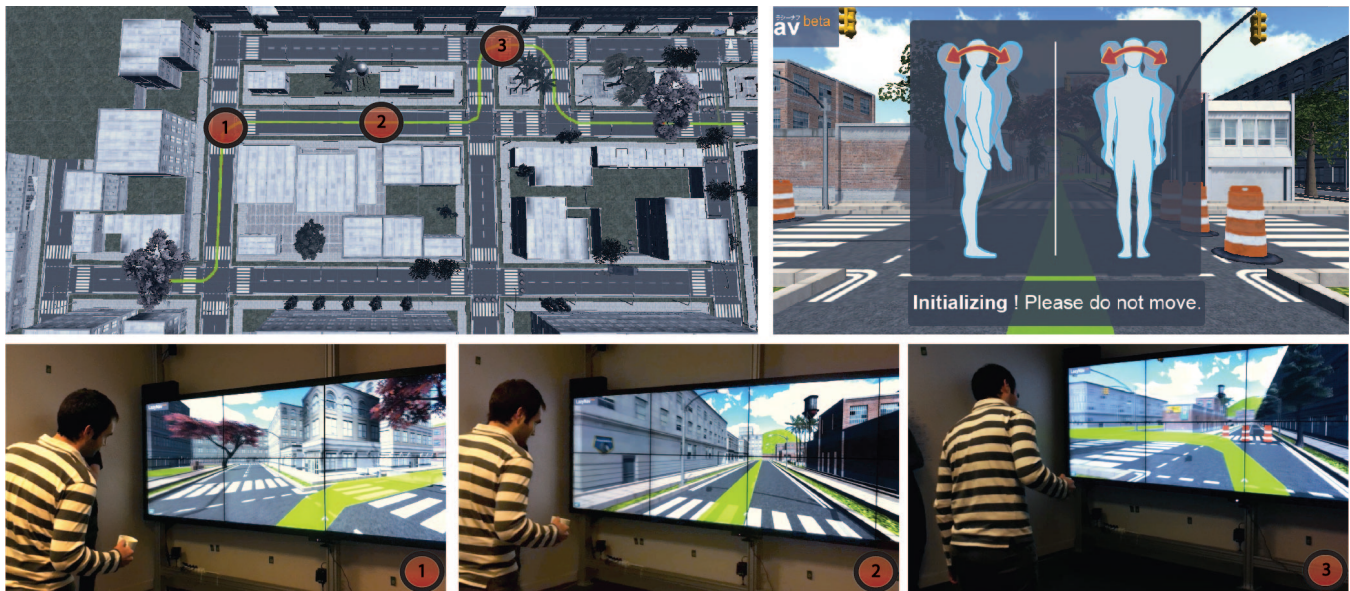
Figure 1: We performed a user study to evaluate several ground navigation metaphors. Top-left: Top view of the virtual city, users have to follow the green path as closely as possible. Top-right: At the beginning of the session, the available motions are displayed to the user, while her rest pose is captured. Bottom: a user is travelling in the scene while holding a cup in his hand.
