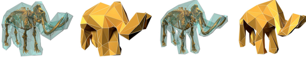
Fig. 16. Comparison with IATV [Mandad et al. 2015]. Left: the input with the IATV mesh in overlay and the mesh alone. Right: the input with our bounding proxy in overlay and the bounding proxy alone. To ensure the strictly enclosing property while using IATV, the input needs to be dilated first, explaining the loss of tightness in the resulting mesh (its volume is 63% higher than ours). Our method performs 20 times faster.
