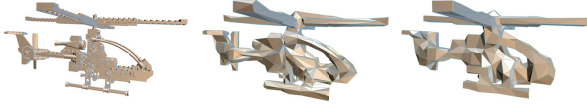
Fig. 9. Meshing. A Lego helicopter (120 components, left), our bounding proxy mesh with a symmetric closing (middle) and with an asymmetric closing (right), which better detects large flat and salient structures.
