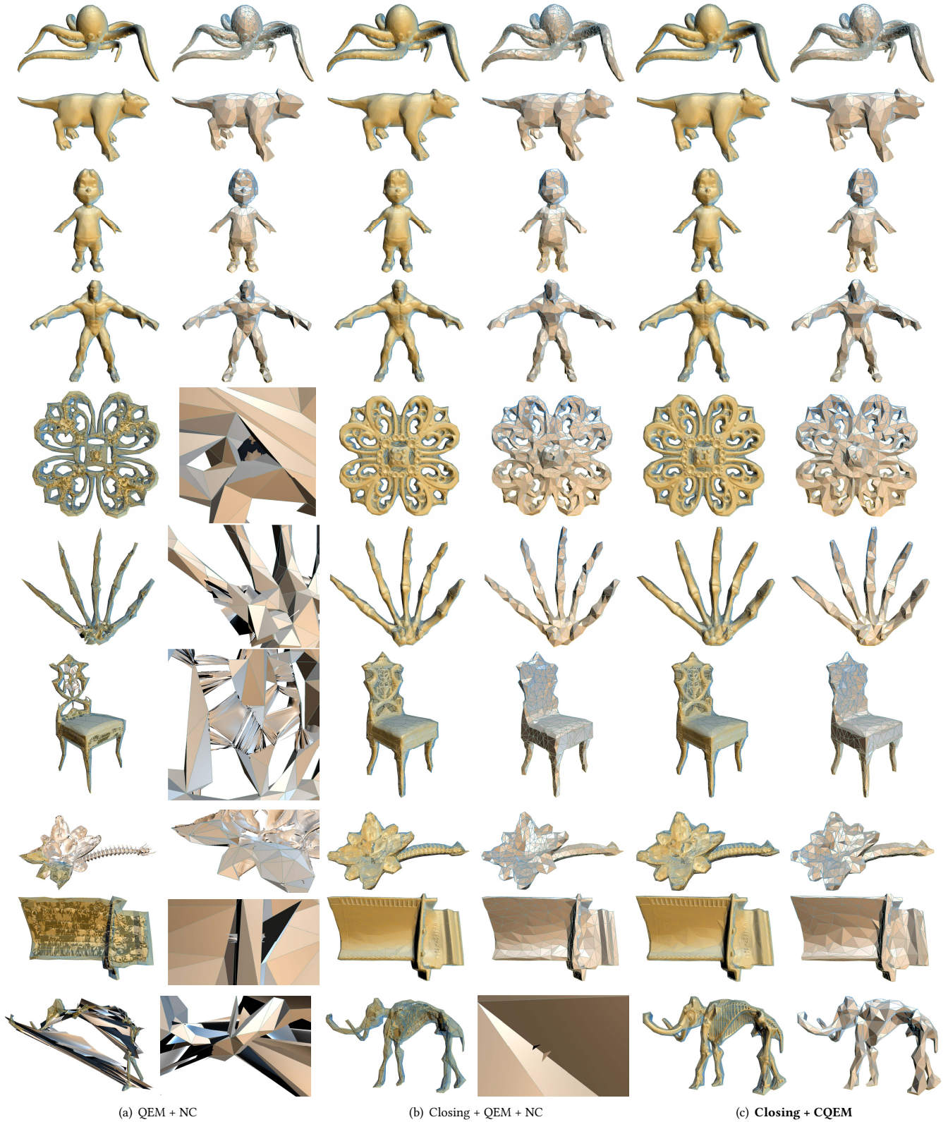
Fig. 14. Comparisons. (a) QEM then Nested Cages. (b) Our closing then QEM then Nested Cages. (c) Our algorithm (closing then CQEM). Closeups are shown in case the Nested Cages shrink flow fails. Quantitative measures are provided in Fig. 13.
